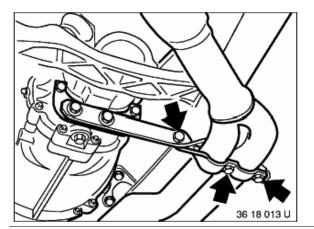
Loosen the bolt connection of the flange on the exhaust manifold.
