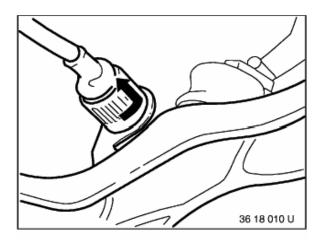
Disconnect connector for oxygen sensor. Unclip the cable from the retainer.
